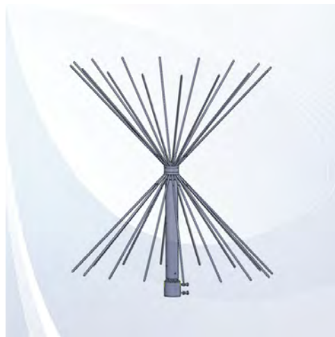
Figure 25.10: A bicone antenna can be thought of as a transmission line with gradually changing characteristic impedance. This enhances impedance matching and the radiation of the antenna (courtesy of antennasproduct.com).
